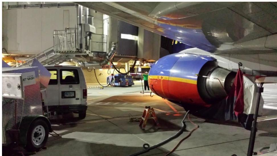
The AJW Wash Unit consists of three tanks: Two 100 Gallon tanks hold pure heated de-ionized water (detergent or alcohol are available if needed) and one 100 Gallon tank holds waste water collected by the Effluent Collection Suit.
