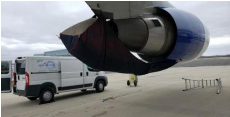
This suit is extremely light, waterproof, and durable which allows for flexible and easy installation, thus reducing the overall wash times.
